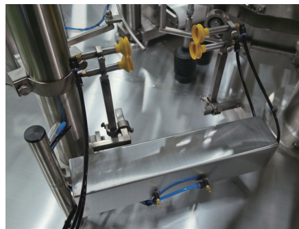
하부벌림장치 Bottom open Stand up opening device
