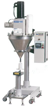
분말충진기(오가필러) Powder Filling Unit (Auger filler)
